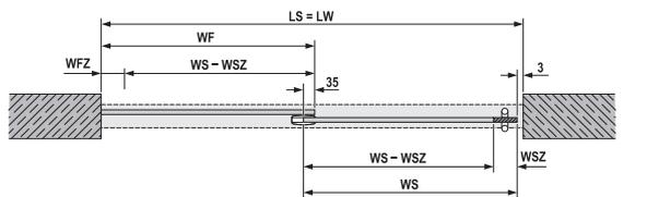
$$WS = \frac{LW - WFZ + WWSZ}{2} + 32 \quad WF = WFZ + WS - WWSZ \quad LS = LW \quad LWt = LW - WF - WWSZ$$
