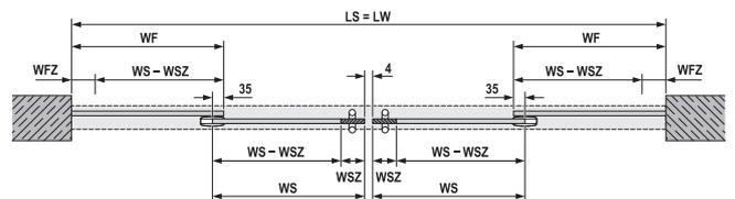
$$WS = \frac{LW - 2WFZ + 2WWSZ + 66}{4} \quad WF = WFZ + WS - WWSZ \quad LS = LW \quad LWt = LW - 2WF - 2WWSZ$$
